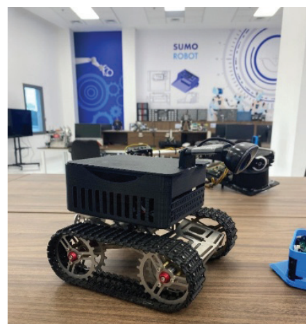
Figure 9: Ground vehicle prototype equipped with a Raspberry Pi 4, motor system, and optical sensing module.
