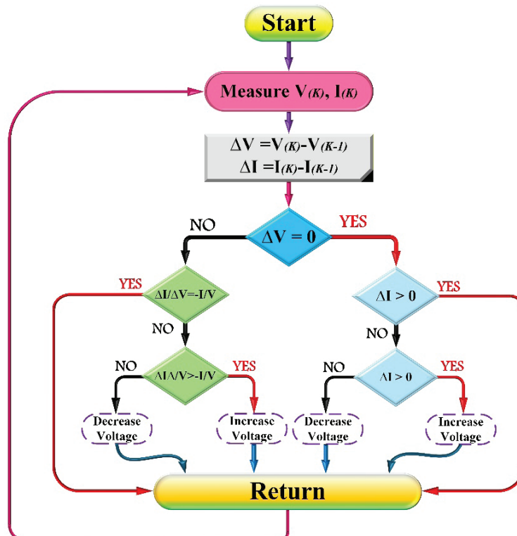
Figure 7: IC algorithm flowchart.
