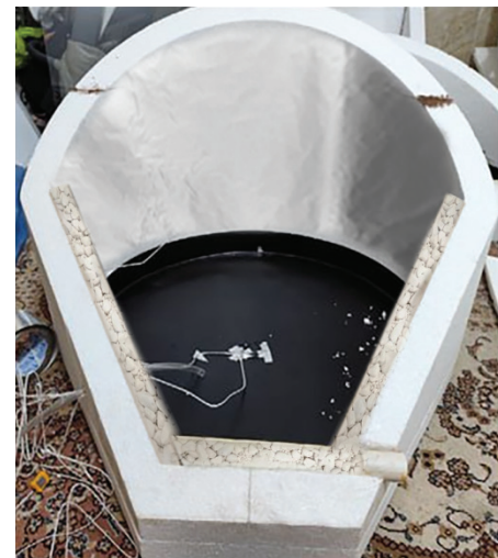
Figure 8: The model is equipped with an enlarged collection channel filled with Thassos stone.
