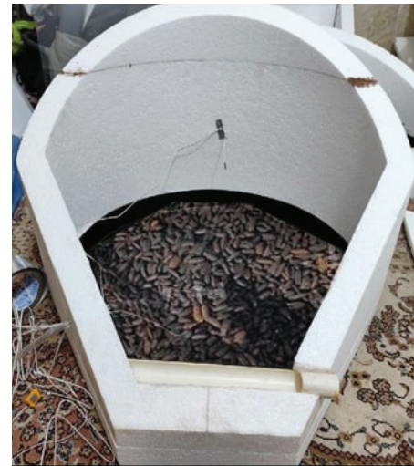
Figure 7: The polygon solar still that uses a layer of burnt date pits.
