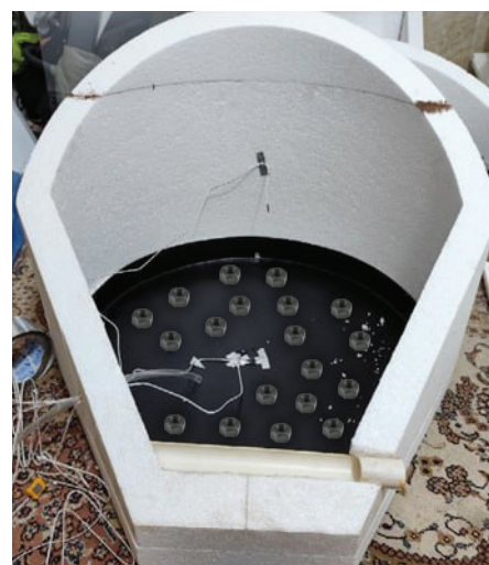
Figure 5: Polygonal solar still enhanced with hexagonal fins.
