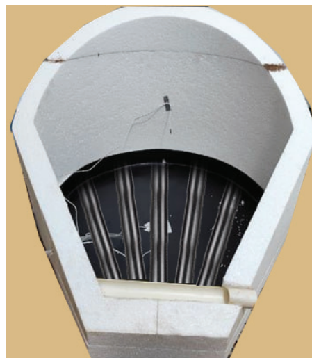
Figure 4: Polygonal solar still enhanced with black-filled heat storage tubes.
