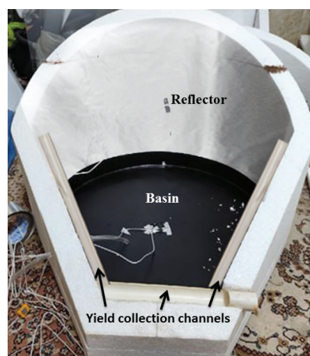
Figure 3: Solar still with internal reflector.
