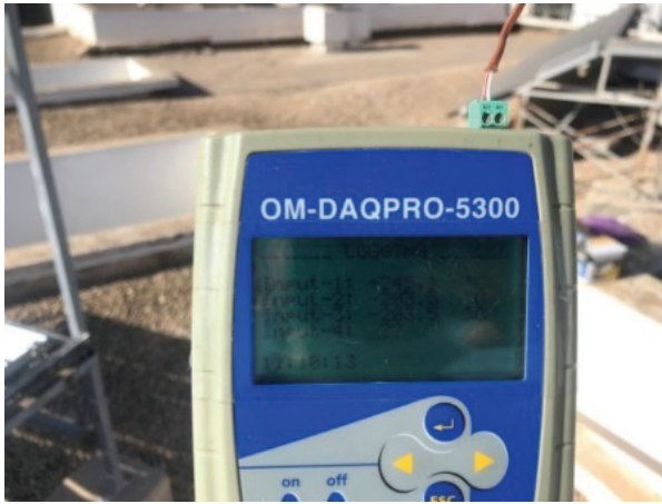
Fig. 9. Picture of the Datalogger « OM-DAQPRO-5300 » used for temperature measurement
