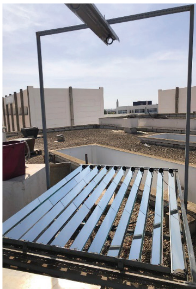
Fig. 3. structure and primary reflector's mirrors
