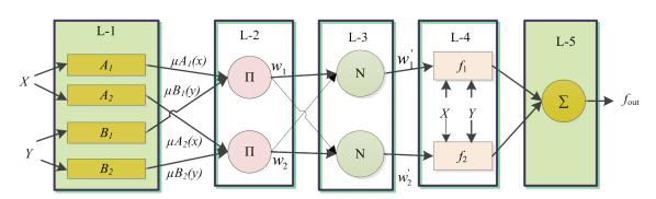
Fig. 5. Functional architecture of ANFIS network
