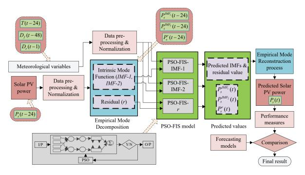
Fig. 7. Evaluation stage of the proposed hybrid EMD-PSO-ANFIS model
