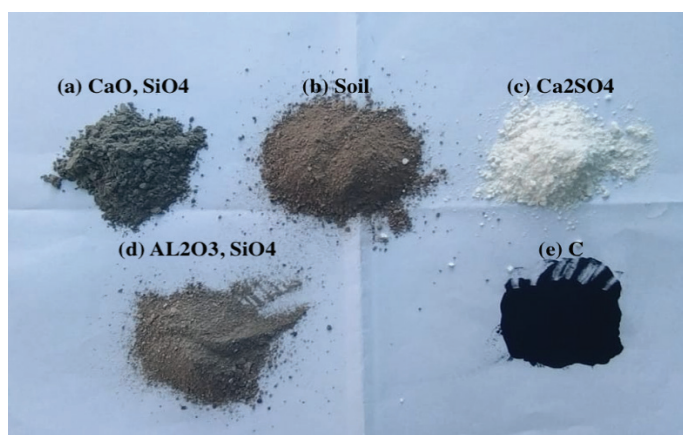
Fig.3. Different Samples of Dust Particles (a) CaO, SiO 4 (b) Soil (c) Ca 2 SO 4 (d) AL 2 O 3 , SiO 4 (e) C
