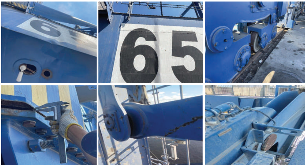
Figure 2: STS12 damage Source: Accident reports
