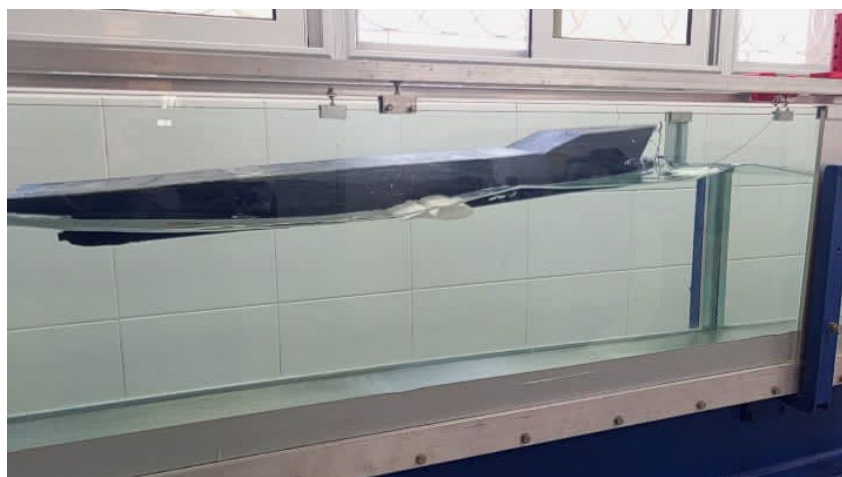
Figure 2: The Printed Model with Attached Fins in Wave Tank.
