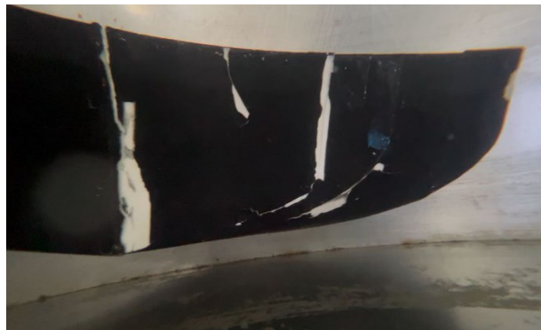
Figure 4: Crack Sample in Pool Environment.
