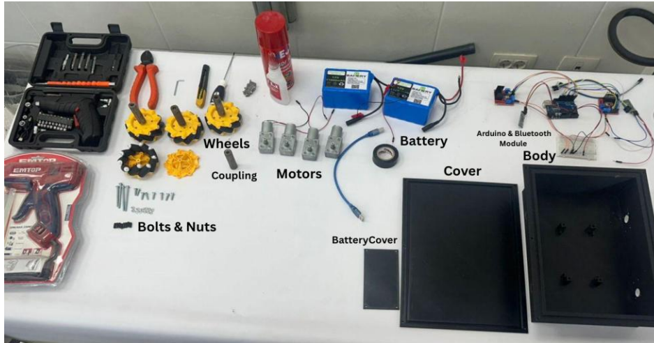
Figure 1: A collection of disassembled robot components on a table, including wheels, tools, batteries, and electronic circuits, for assembly
