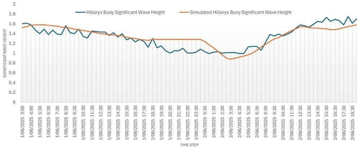
Figure 17: Simulated Hs and the recorded Hs by Hillarys buoy, located at Lat - 31.852°, Long 115.647° WGS 84
