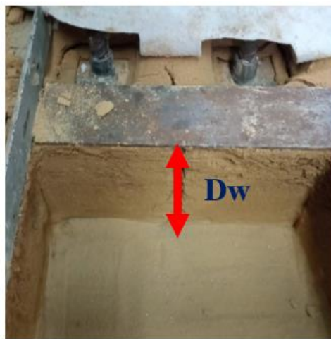
Figure (5): The depth of wetting ( D_w ) beneath the footing center [ \gamma_d = 14.41 \text{ kN/m}^3 , F=76.62\% , B=7.6 \text{ cm} , W_o=3.6\% , q=100 \text{ KN/m}^2 , N=4 , Q_w=3 \text{ cm}^3/\text{cm}^2 ].
