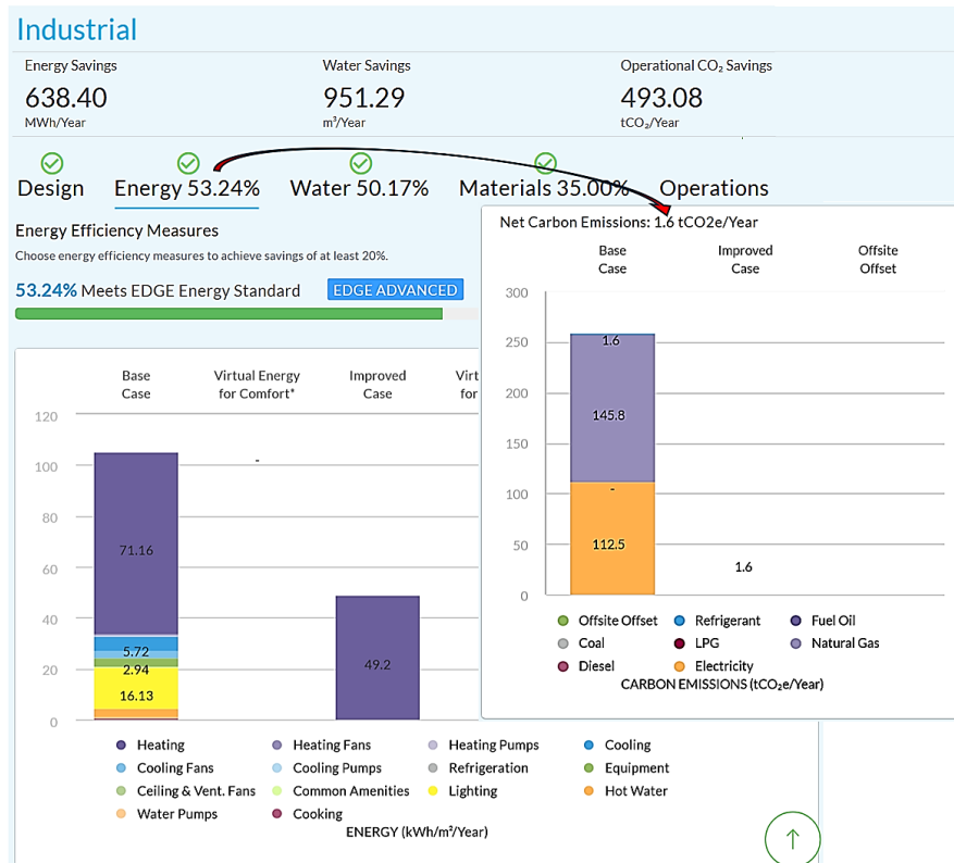
Figure 7. Print Screen of the results after replacing the lighting and hot water systems and installing the PV plant
