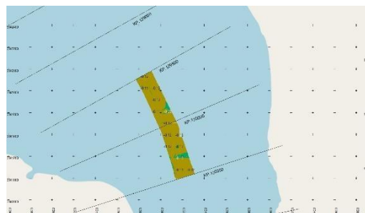
Figure 9: Differential chart illustrating the disparities between RTK tide data and tide gauge data for the second experimental 10 km, PDS 2000.
