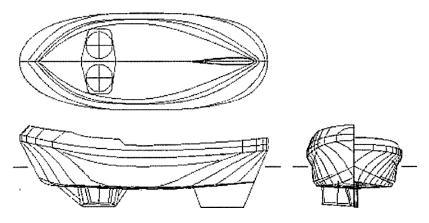
Figure 3: Lines of AJAX hull
