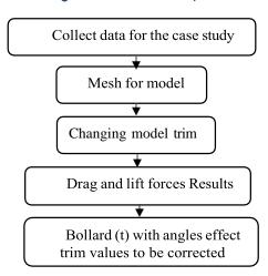
In this study, a 1:18 scale model of Ajax without a tug appendage was used to create a full-size model of the Escort tug. Table 1 (4) contains the model's primary characteristics. A speed of (0.2, 0.4, 0.6, 0.8, 1, 1.2, 1.4) m/s was employed in the current study.
