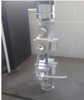
Figure 4: Tensile test setting.
