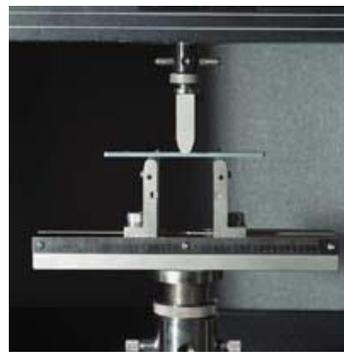
Figure 5: Bending test setting.
