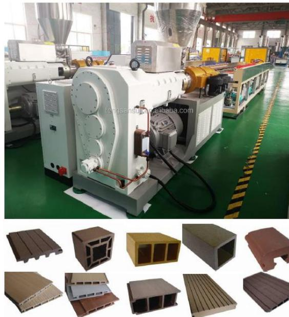
Figure 3: Conical double screw extruder.
