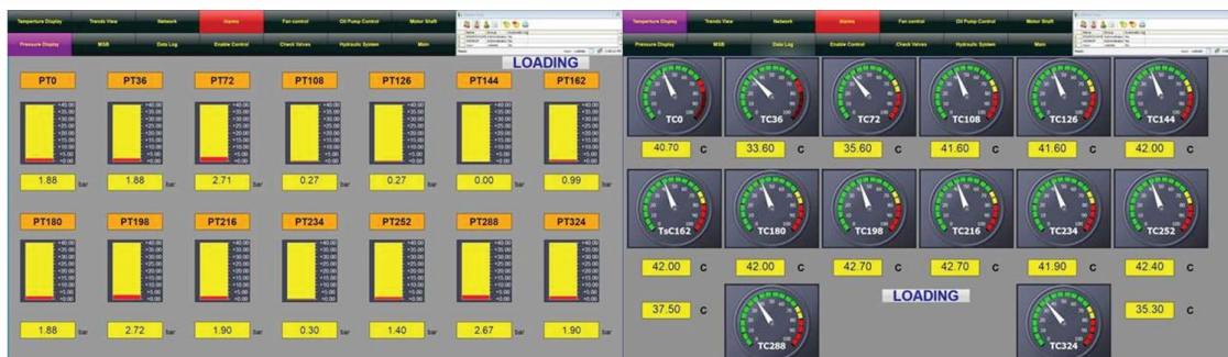
Oil Film Pressure Distribution Display Page
