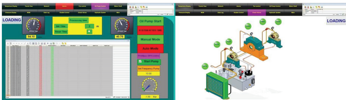
Main Lubricating Oil Pump Control Page
