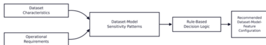
Figure 12: IDS-ReComm workflow: dataset characteristics and operational requirements combine with empirically derived dataset-model sensitivity patterns and rule-based decision logic to produce configuration recommendations.
