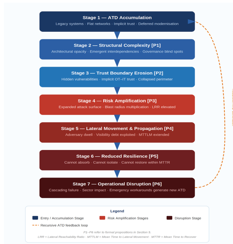
Figure 2: ATD-Induced Systemic Cyber Risk Model. Seven-stage causal chain from ATD accumulation (Stage 1) to operational disruption and recursive debt generation (Stage 7). Stages reference the formal propositions P1–P6 (Section 5).
