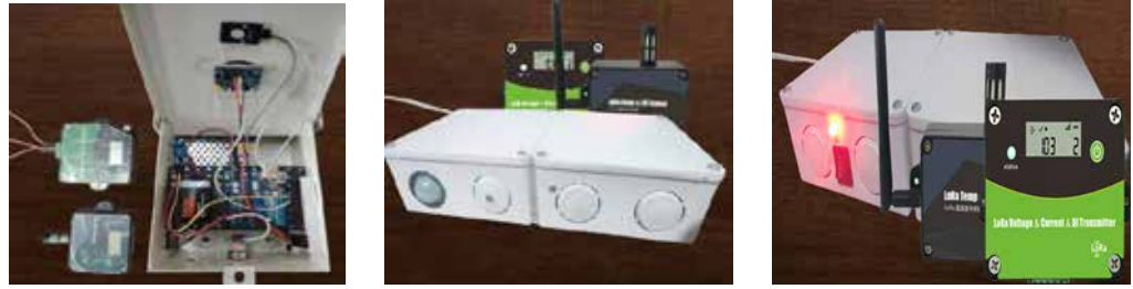
Figure 2: (Box) Set of sensors for each station deployed at MOST-BARMM: (a) Open top view showing hardware inside; (b) Front-side view with PIR, LoRa temp/humidity sensors, and UV light sensors; (c) Back-side view with system switch and pilot light
