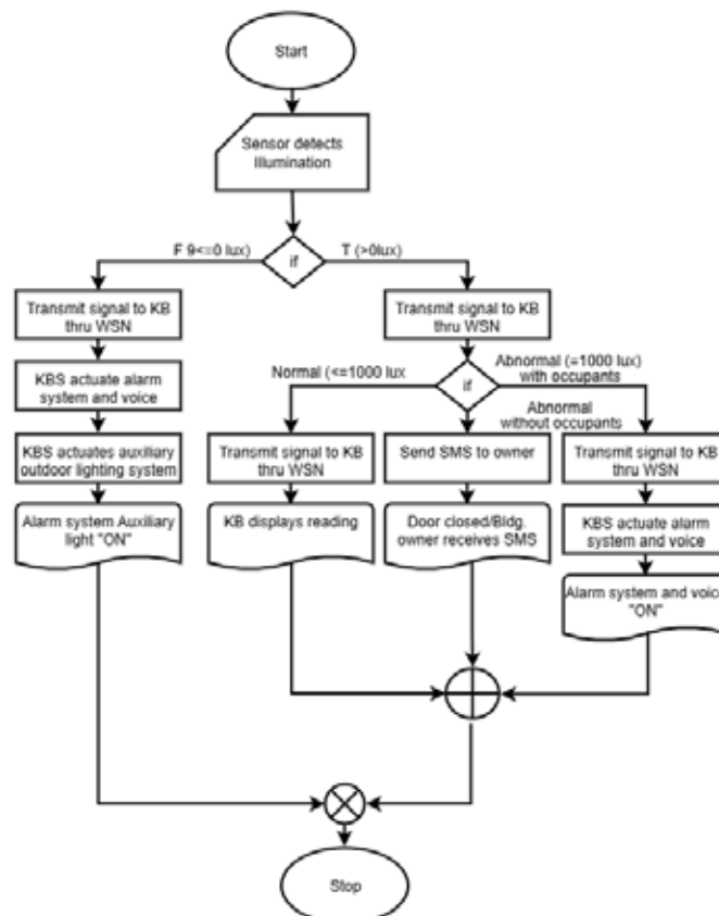
Figure B-8: Algorithm for Light Sensor Night Operation
