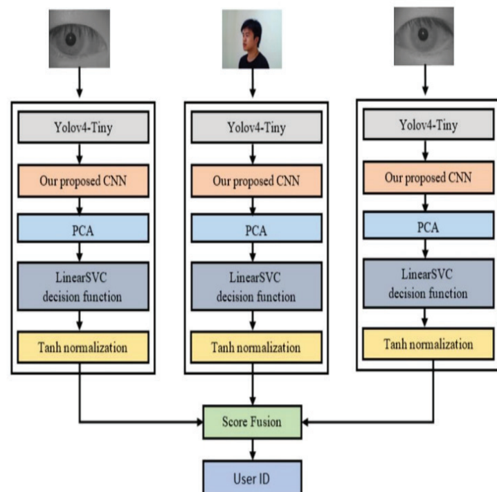
Figure 2: Face-iris recognition system based on score-level fusion
