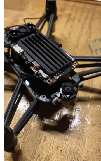
Figure 7: Modified drone prototype with a repositioned downward-facing camera to enable vertical image capture for YOLO-based detection.
