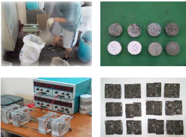
Fig .2. Procedure of rapid chloride penetration test
