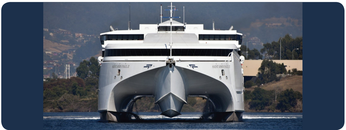
Fig. 4. The new centrebow design of Saint John Paul II, Incat catamaran, length overall = 110m. (Swidan et al., 2019). Note: that all Incat manufactured vessels had previously a smooth centrebow without any appendages for water separation during water-entry and to enhance her vessels' seakeeping performance.
