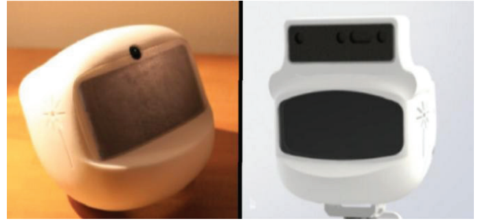
Figure 7. shows the Poppy head design (left) while the RAFEQI head design (right) [7]
