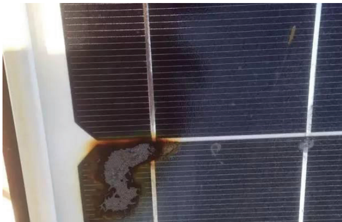
Fig. 5. Soldering defects in solar cells
