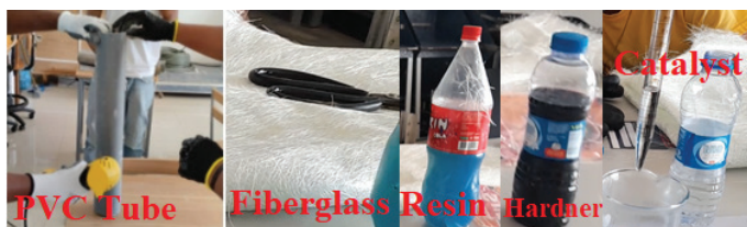
Fig. 4. Materials used for constructing the Wells turbines
