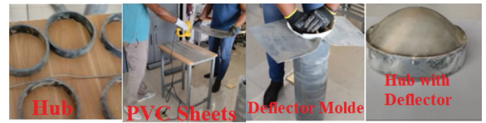
Fig. 5. Construction of the Wells turbine hubs and deflectors
