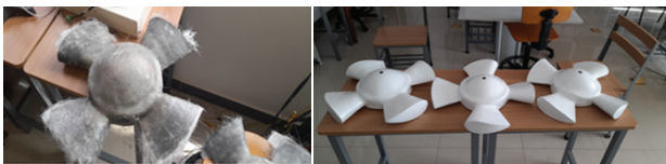
Fig. 9. Fibreglassing and finishing of the Wells turbines
