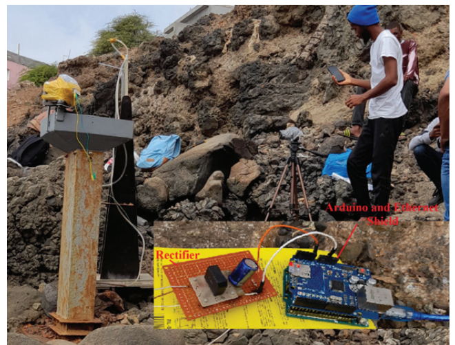
Fig. 3. Experimental setup to study the MNC production when equipped with the Wells turbine
