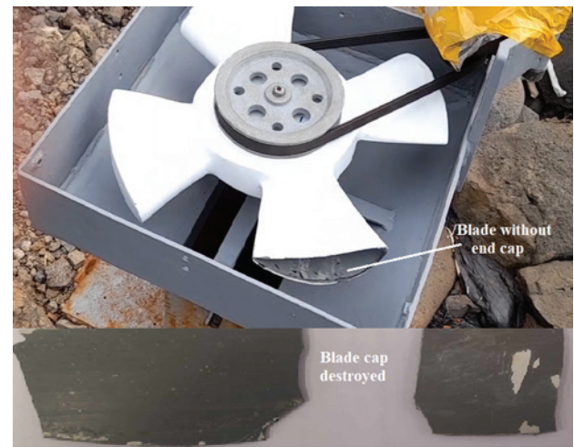
Fig. 30. Blade cap destroyed by centrifugal force
