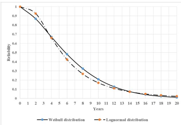
Fig. 3 Reliability of different probability distributions for 500 kV subpopulation
