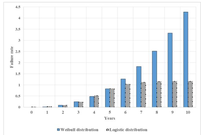
Fig. 8 Failure rates of different probability distributions for 66-33 kV subpopulation.
