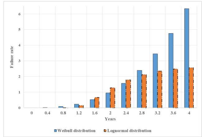
Fig. 4 Failure rates of different probability distributions for 220 kV subpopulation
