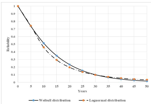
Fig. 7 Reliability of different probability distributions for 132 kV subpopulation.
