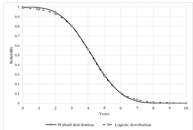
Fig. 9 Reliability of different probability distributions for 66-33 kV subpopulation.
