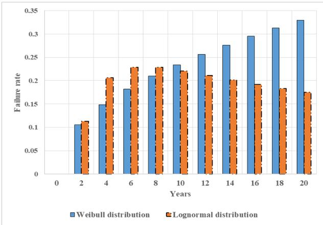
Fig. 2 Failure rates of different probability distributions for 500 kV subpopulation
