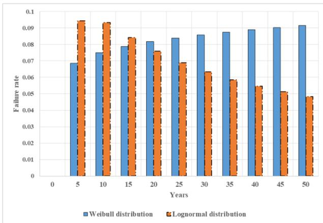
Fig. 6 Failure rates of different probability distributions for 132 kV subpopulation.
