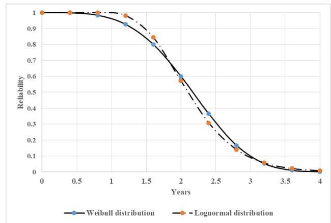
Fig. 5 Reliability of different probability distributions for 220 kV subpopulation
