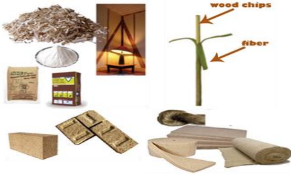
Fig.1. Shows Hemp wood chips are mixed with lime to create hempcrete Bricks and insulation sheets
