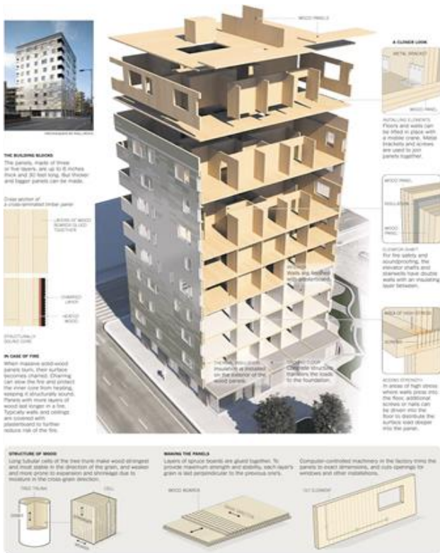
Fig.8. Shows the wood structure of the 9 stores Stadthaus, Murray Grove residential building.
