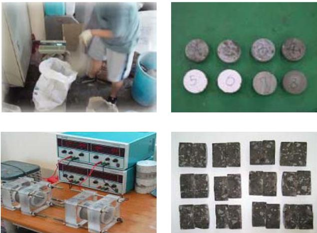
Fig .2. Procedure of rapid chloride penetration test
