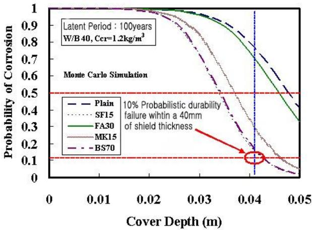
Fig.10. Durability failure possibility according to shield thickness
