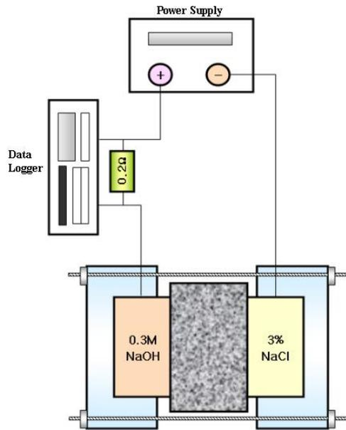
Fig .1. Diagram of chloride ion diffusion test equipment
