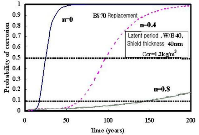
Fig. 7. Durability failure possibilities according to the time dependent coefficient
