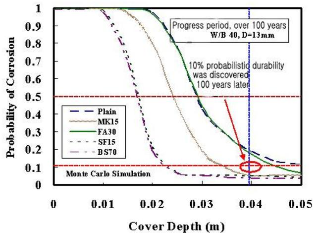
Fig.13. Durability failure possibility according to shield thickness
