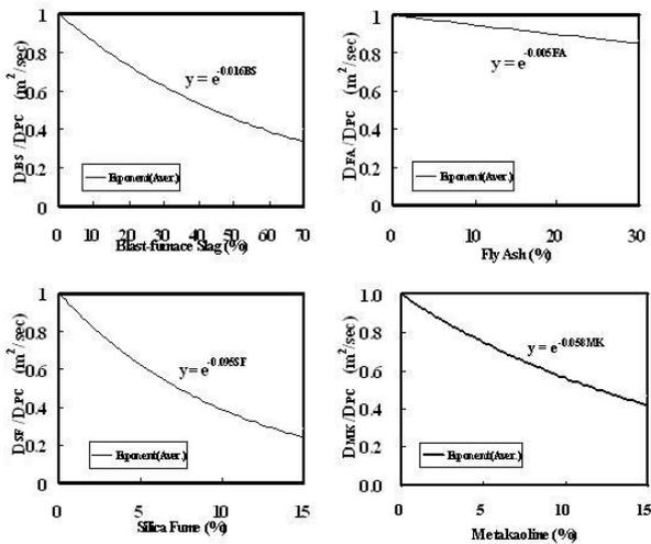
Fig. 6. Type of admixture and substitution ratio
