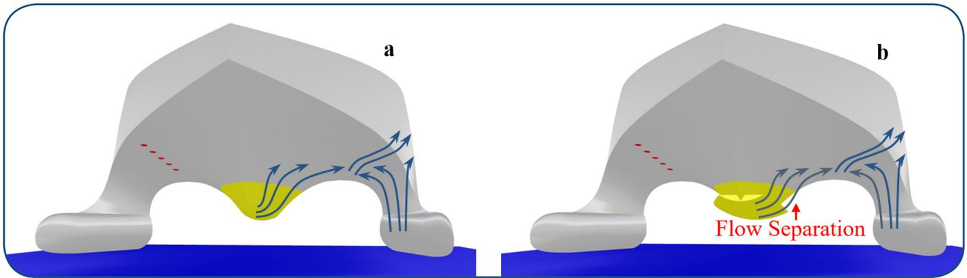
Fig. 3. Schematic drawing showing the expected low behaviour on one side during water penetration of; (a) parent centrebow and (b) amended centrebow (Swidan et al. (2016b)).
