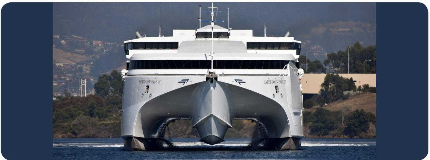
Fig. 4. The new centrebow design of Saint John Paul II, Incat catamaran, length overall = 110m. (Swidan et al., 2019). Note: that all Incat manufactured vessels had previously a smooth centrebow without any appendages for water separation during water-entry and to enhance her vessels' seakeeping performance.
