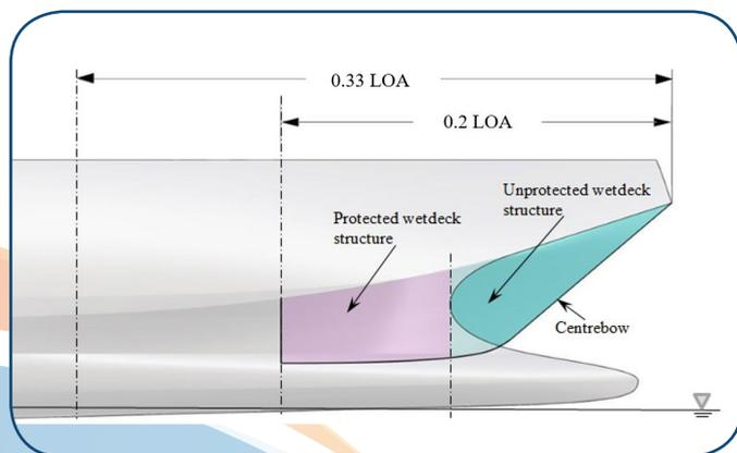
Fig. 1. Schematic diagram of bow section for a catamaran.
