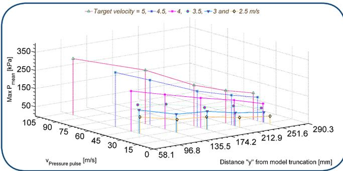
Fig. 6. 3-d plot showing the effect of the transducer location on both the peak slam pressures and the corresponding pressure pulse velocities (vy) in the "y" direction in relation to six water impact velocities. The x-scale presents the longitudinal locations of the five pressure transducers against the y-scale that presents the range of the calculated mean vy and the z-scale that presents the mean slam peak pressures of 26 tests.
