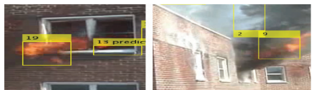
Fig. 3. Samples of fire detection outside the building.
