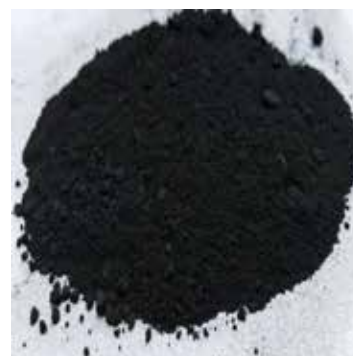
Fig. 2. Biochar prepared by firing in Nitrogen to 600°C
