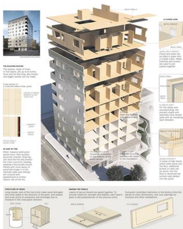
Fig.8. Shows the wood structure of the 9 stores Stadthaus, Murray Grove residential building.
