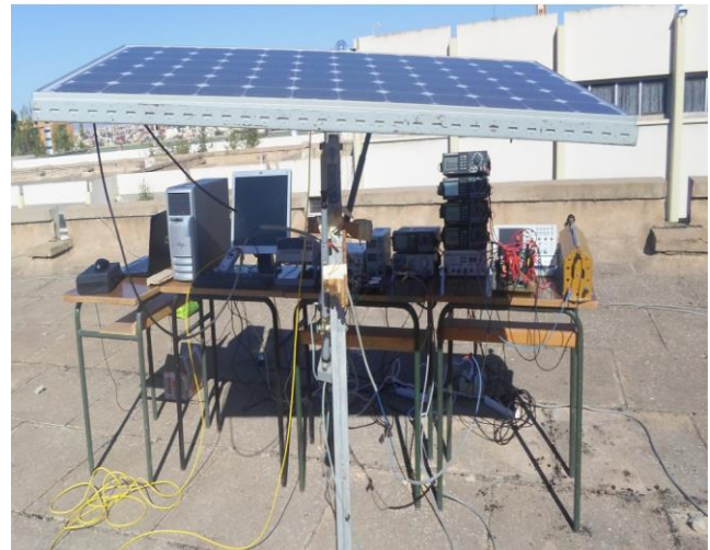
Fig .4. Bench of automated measurements, prototype photovoltaic (panels, tracker of the sun, Converter Boost MPPT command).
