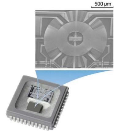
Silicon Micromachined Gyro for Application in Navigation Systems.
